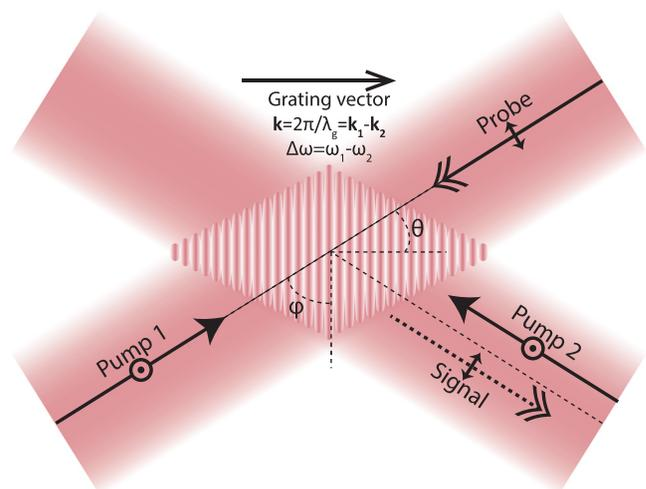
FIG. 1. Schematic of a typical CRBS geometry. Two almost counter-propagating, equipolarized pump beams cross within a medium at a half-angle  $\phi$  to create an optical lattice. A probe beam, normally polarized to the pumps, is incident at this lattice at the Bragg angle  $\theta$  and is being scattered from it producing a signal beam, which maintains all the spatial and polarization characteristics of the probe beam.
